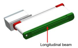
2. Disassemble mounting beams (marked in green - see illustration)
