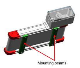
Move belt on the lower side of the transport body to the side and loosen the set screws on one side of the cross beam (marked in green - see illustration)
